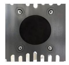
The picture illustrates the visual difference between two different absorber coatings. The outer plate is an  $\alpha C$  coating with R~13% and the plate in the middle is an absorber coating with R~0.2% coated by Polyteknik AS.
